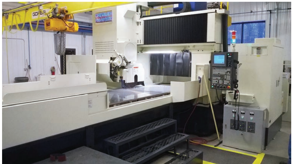
The Chevalier FSG-50120DC can obtain parallelism of .0002" across the entire distance.
